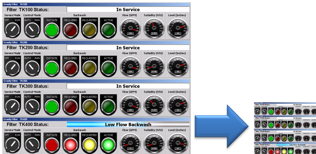
Figure 2: Shrinking bitmaps in InTouch does not decrease the size on disk, and rendering takes the same amount of time as the bitmap at full size.
